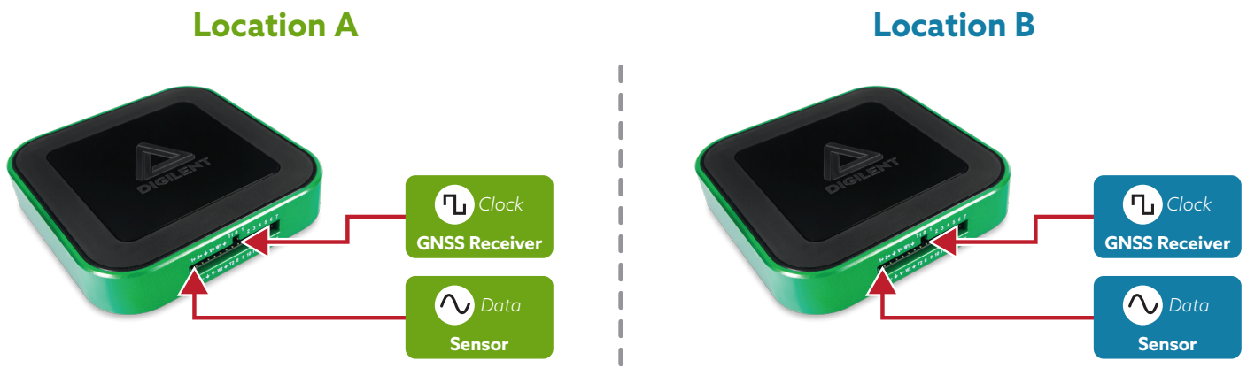
Figure 4: GPS synchronization for physically separated acquisition sites
